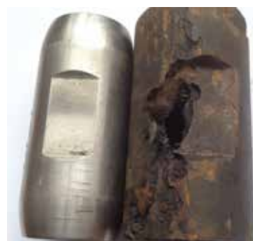
Figure 3. EH9 coupling (after 280 days) vs. T coupling (after 180 days)
