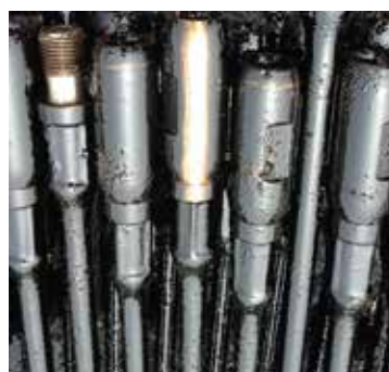
Figure 3. EH9 rod shows no visible corrosion after 280 days of operation
